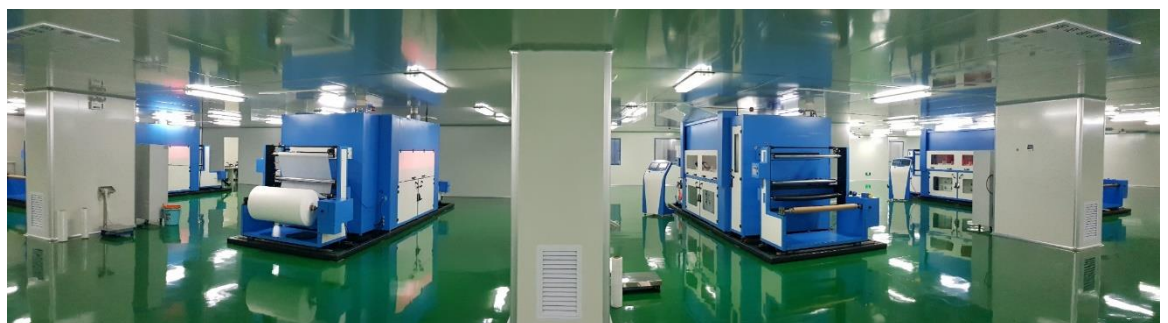
Industrial Nanofiber Production Line (One stop service): yield of 4-20 g/hr. upto 100 g/hr., nanofiber sizes of 60-500 nm.
